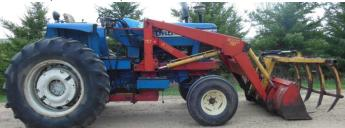
•Ford 6700 tractor w/ Leon 707 FEL & 6 ft. bucket & grapple, 75 hp., 2WD, 9,347 hours showing, 3 pt. hitch, 2 hyd's, 18.4 X 34 tires.
