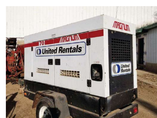
Magnum 70kw Generator
