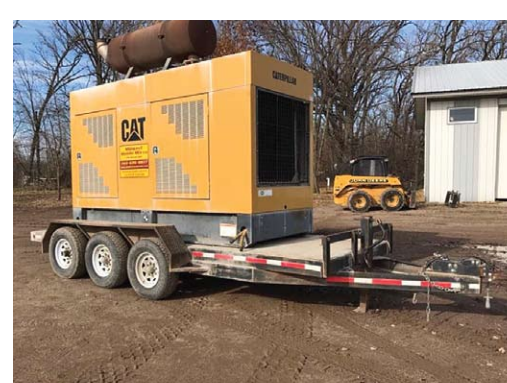
Caterpillar 365kw Generator
