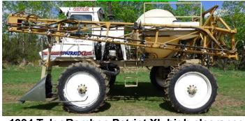
•1994 Tyler Ramboc Patriot XL high clearance 75' sprayer, 800 gal. poly tank, GPS for steering & flow control, 2,662 hours, crop dividers, rinse tank, JD 4 cyl. diesel, susp. front folding booms, 3-way nozzle bodies, 20" nozzle spacing.
