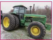
Diesel Tractor, Sound Guard Cab, Power Shift, 18.4R X 42 Inch
