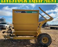
Vermeer BP8000 Bale Processor, twine cutter, 16" flotation tires, 1000 PTO, rear bale carrier, left hand unload, like new!
