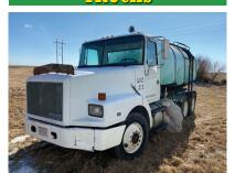
1990 White/GMC Conventional Truck, Cummins diesel, 9-spd., 11r22.5 tires, 3.000-gal. fertilizer tank, with Honda gas engine & pump GMC 6000 Fuel Truck, V-8, 5-speed, 2,500-gal.
