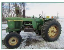
1966 John Deere Model 4020 Diesel Tractor, Open Station, Synchro, Differential Lock, Front Side Weights, 540/1000 PTO, John Deere Wide Front and 3-Point, 18.4 X 34 Inch Tires, 18.4 X 34 Inch Band Duals, Ser. #SNT213R123539R
