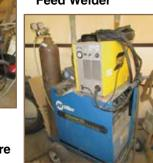
Miller Syncrowave 250 AC DC 220V Single Phase Wire **Feed Welder**
